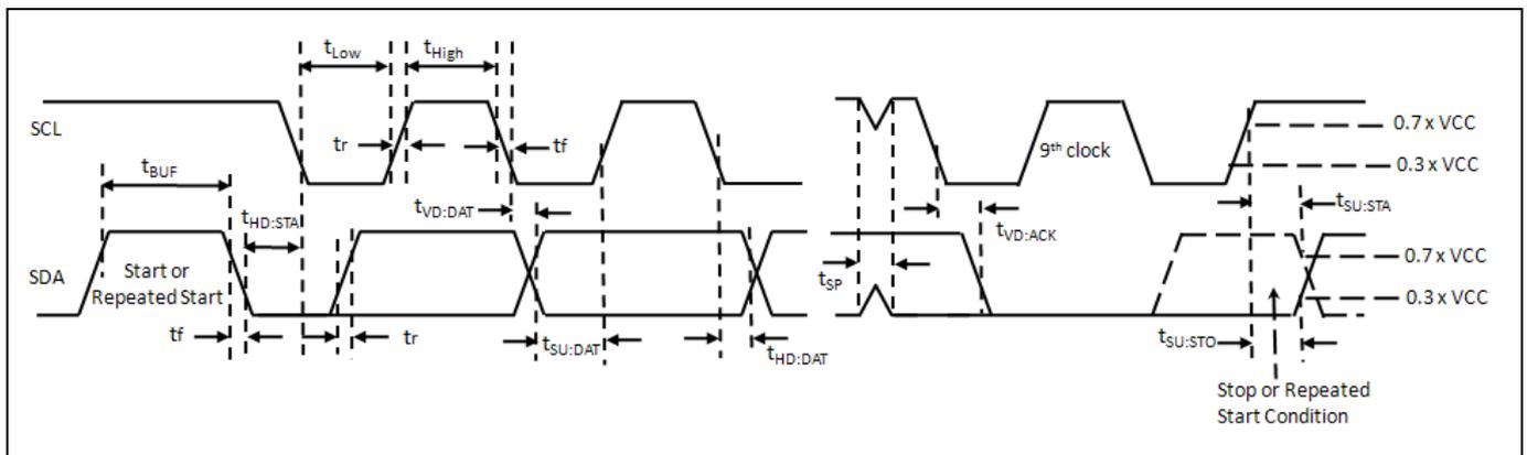
**Figure 2. Definition of Timing on the I2C-bus**
