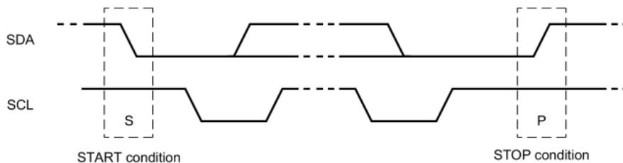
**Figure 8. Definition of Start and Stop Conditions**
