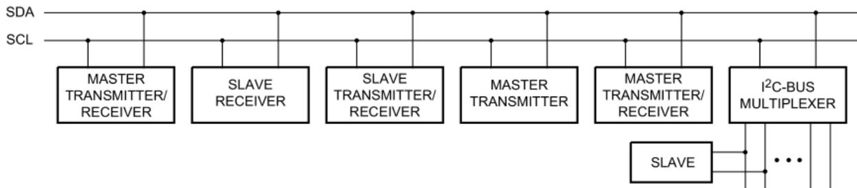
**Figure 9. System Configuration**
