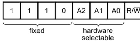
Figure 4. Device Address
