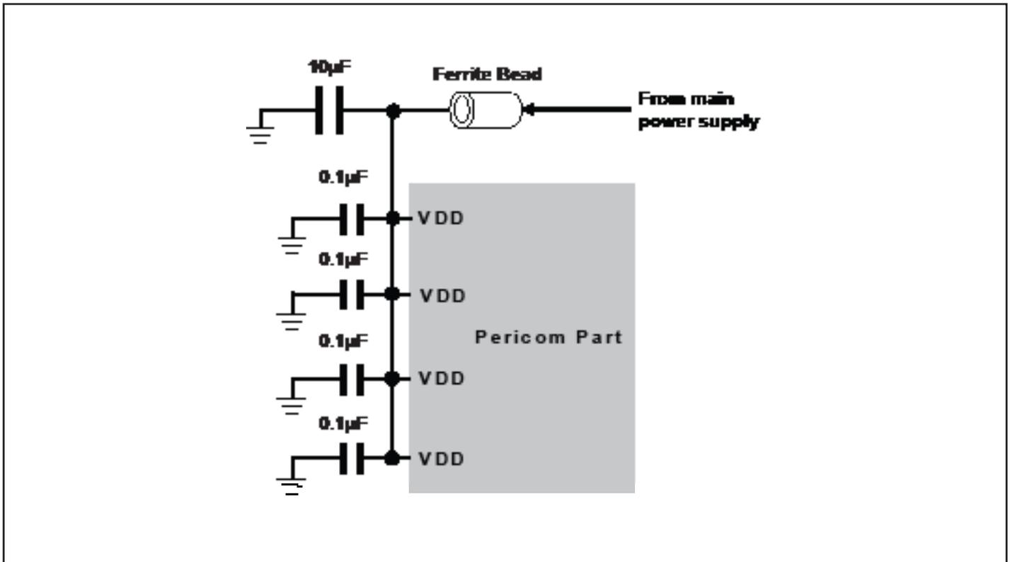
**Figure 1 Recommended Power Supply Decoupling Circuit Diagram**
