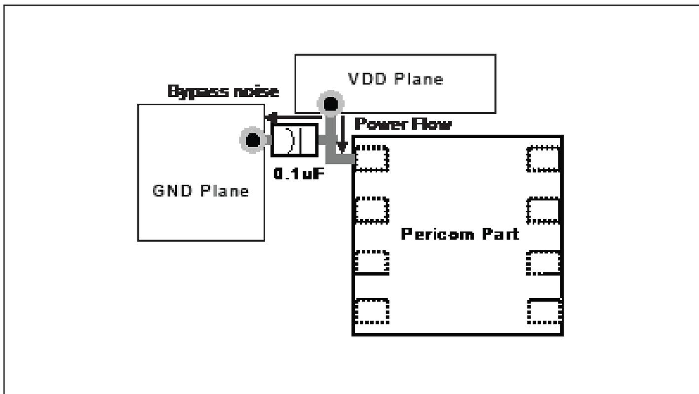
**Figure 2 Layout and Decoupling Capacitor Placement Diagram**
