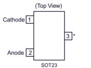
\* Pin 3 must be left floating or connected to pin 2
