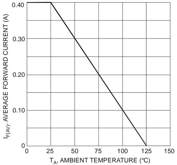
Fig. 4 Forward Current Derating Curve, Per Element
