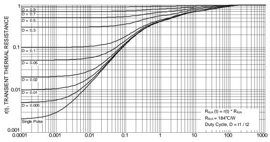
t1, PULSE DURATION TIME (sec) Figure 14 Transient Thermal Resistance
