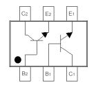
Device Schematic and Pin-Out Top View
