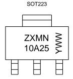
ZXMN 10A25 = Product Type Marking Code YWW = Date Code Marking Y or  $\overline{Y}$  = Last Digit of Year (ex: 2= 2022) WW or  $\overline{W}W$  = Week Code (01~53)
