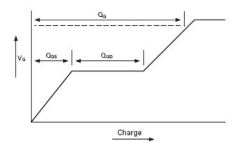
Basic gate charge waveform
