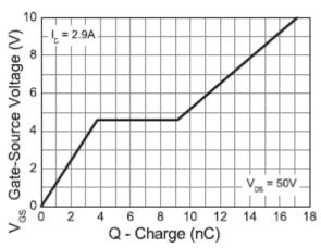
Gate-Source Voltage v Gate Charge
