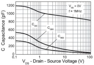
Capacitance v Drain-Source Voltage
