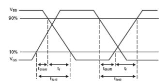
Switching time waveforms
