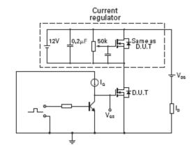
Gate charge test circuit
