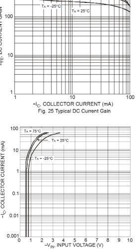
Fig. 27 Typical Collector Current vs. Input Voltage
