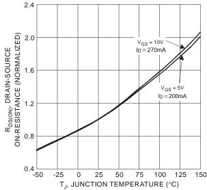
Figure 5 On-Resistance Variation with Temperature
