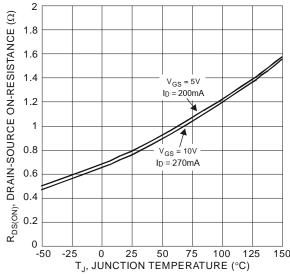
Figure 6 On-Resistance Variation with Temperature
