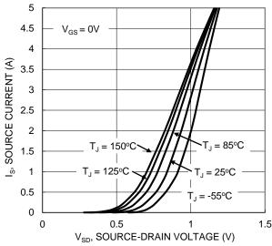
Figure 9. Diode Forward Voltage vs. Current
