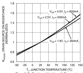
Figure 6. On-Resistance Variation with Temperature
