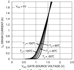
Figure 2. Typical Transfer Characteristic
