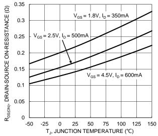
Figure 7. On-Resistance Variation with Temperature
