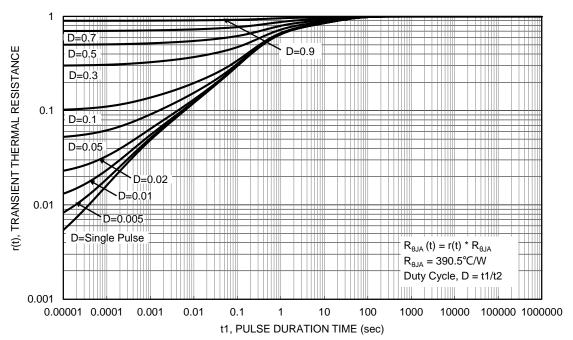
Figure 13. Transient Thermal Resistance
