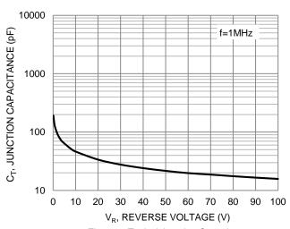
Figure 3. Typical Junction Capacitance
