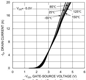
Figure 2. Typical Transfer Characteristic
