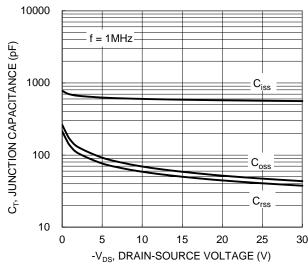
Figure 10. Typical Junction Capacitance
