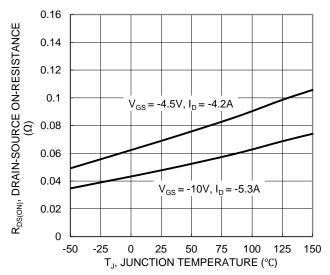
Figure 7. On-Resistance Variation with Temperature
