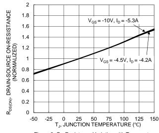
Figure 6. On-Resistance Variation with Temperature
