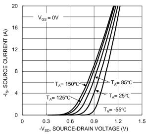
Figure 9. Diode Forward Voltage vs. Current
