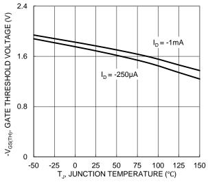
Figure 8. Gate Threshold Variation vs. JunctionTemperature
