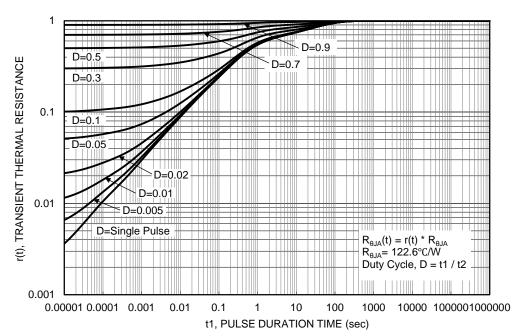
Figure 13. Transient Thermal Resistance
