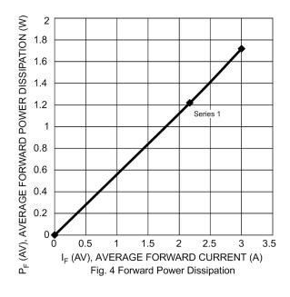
Notes: 7. Device mounted on FR-4 substrate, 0.4"\*0.5", 2oz, single-sided, PC boards with 0.2"\*0.25" copper pad. 8. Device mounted on FR-4 substrate, 1"\*1", 2oz, single-sided, PC boards with 0.06"\*0.09" copper pad.
