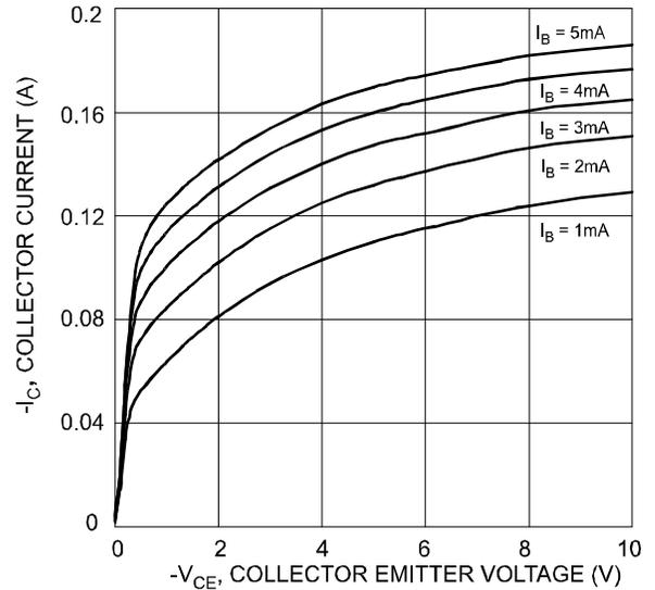
Fig. 2 Typical Collector Current vs. Collector Emitter Voltage
