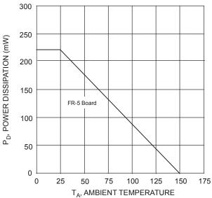
Fig. 4 Steady State Power Derating Curve
