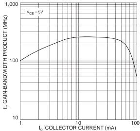
Figure 3 Gain-Bandwidth Product vs Collector Current
