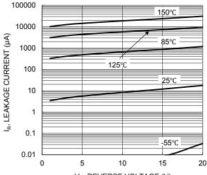
$V_R$ , REVERSE VOLTAGE (V) Figure 2. Typical Reverse Characteristics
