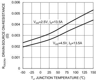
Figure 7. On-Resistance Variation with Junction Temperature
