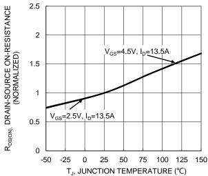
Figure 6. On-Resistance Variation with Junction Temperature
