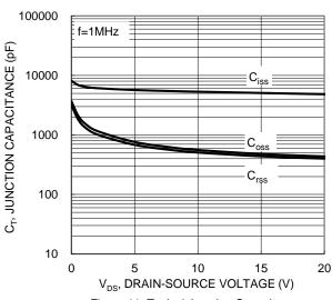
Figure 11. Typical Junction Capacitance
