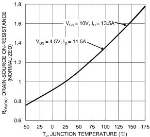
Figure 6. On-Resistance Variation with Junction Temperature
