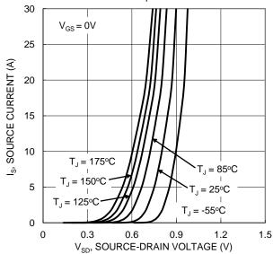
Figure 9. Diode Forward Voltage vs. Current
