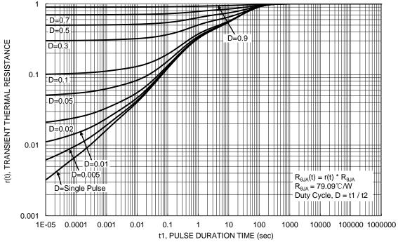
Figure 13. Transient Thermal Resistance
