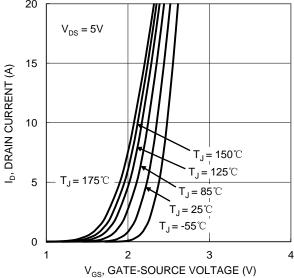
Figure 2. Typical Transfer Characteristic
