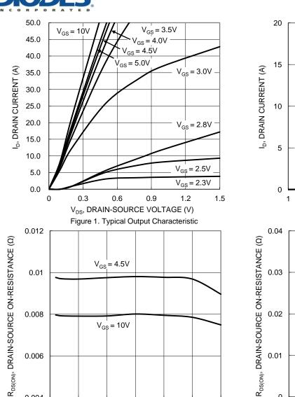
I<sub>D</sub>, DRAIN-SOURCE CURRENT (A) Figure 3. Typical On-Resistance vs. Drain Current and Gate Voltage
