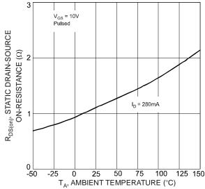
Fig. 7 Static Drain-Source On-State Resistance vs. Ambient Temperature
