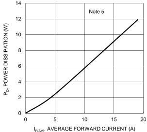
Figure 1. Forward Power Dissipation
