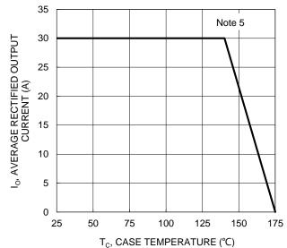
Figure 4. DC Forward Current Derating
