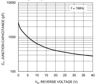
Figure 5. Typical Junction Capacitance
