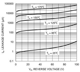
Figure 3. Typical Reverse Characteristics
