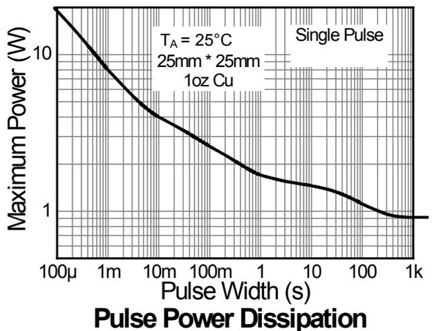
**Typical Electrical Characteristics** (@ $T_A = +25^\circ\text{C}$ , unless otherwise specified.) (continued)
