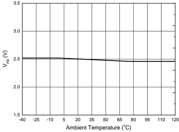
**V<sub>BP\_HVON</sub> Voltage vs. Ambient Temperature**
