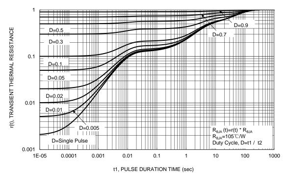
Figure 25. Transient Thermal Resistance
