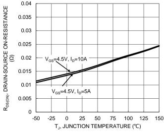
Figure 7. On-Resistance Variation with Temperature
