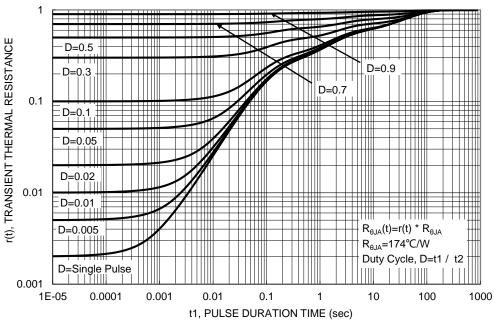
Figure 14. Transient Thermal Resistance
