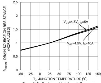
Figure 6. On-Resistance Variation with Temperature
