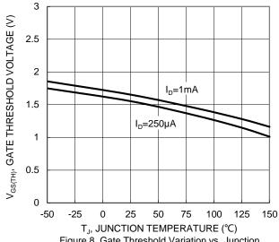
Figure 8. Gate Threshold Variation vs. Junction Temperature
