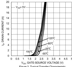
Figure 2. Typical Transfer Characteristic
