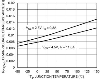
Figure 7. On-Resistance Variation with Junction Temperature
