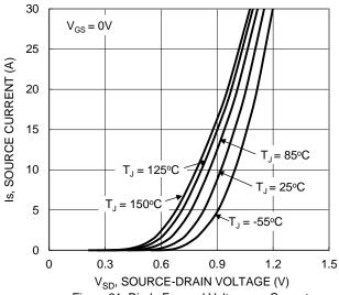
Figure 21. Diode Forward Voltage vs. Current
