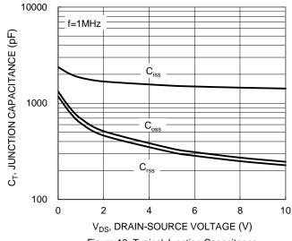
Figure 10. Typical Junction Capacitance
