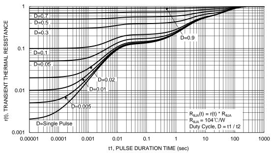
Figure 25. Transient Thermal Resistance
