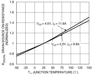
Figure 6. On-Resistance Variation with Junction
