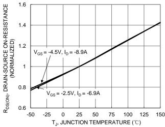
Figure 18. On-Resistance Variation with Junction Temperature
