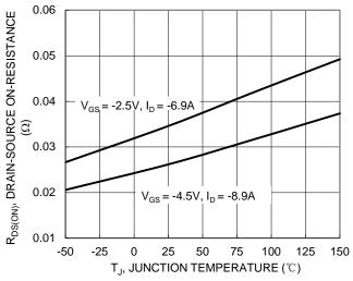
Figure 19. On-Resistance Variation with Junction Temperature
