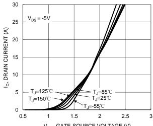
V<sub>GS</sub>, GATE-SOURCE VOLTAGE (V) Figure 14. Typical Transfer Characteristic
