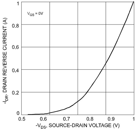
Fig. 18 Drain Reverse Current vs. Source-Drain Voltage
