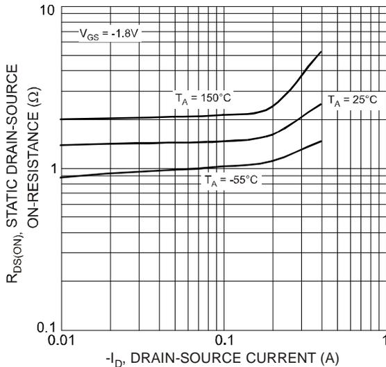
Fig. 15 Static Drain-Source On-Resistance vs. Drain Current
