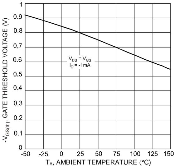
Fig. 13 Gate Threshold Voltage vs. Ambient Temperature
