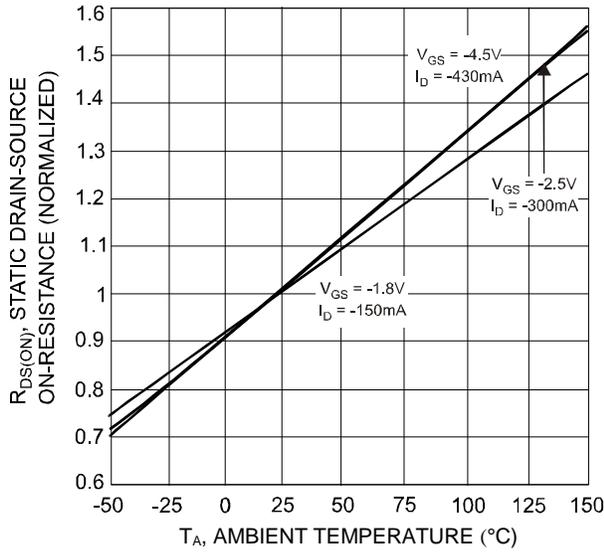
Fig. 17 Static Drain-Source On-State Resistance vs. Ambient Temperature
