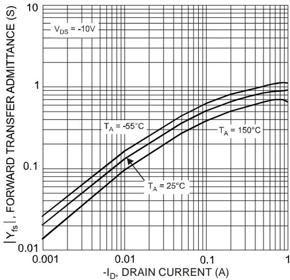
Fig. 19 Forward Transfer Admittance vs. Drain Current
