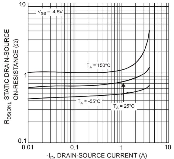
Fig. 14 Static Drain-Source On-Resistance vs. Drain Current
