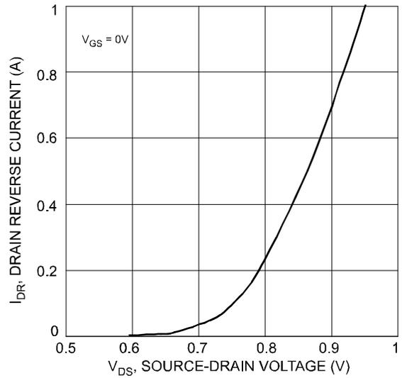
Fig. 8 Drain Reverse Current vs. Source-Drain Voltage
