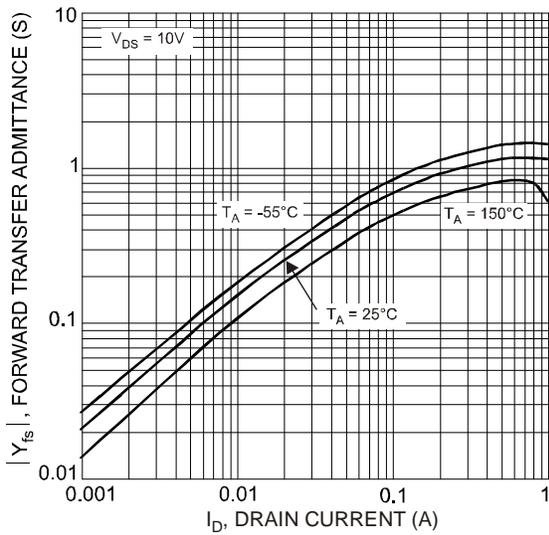
Fig. 9 Forward Transfer Admittance vs. Drain Current
