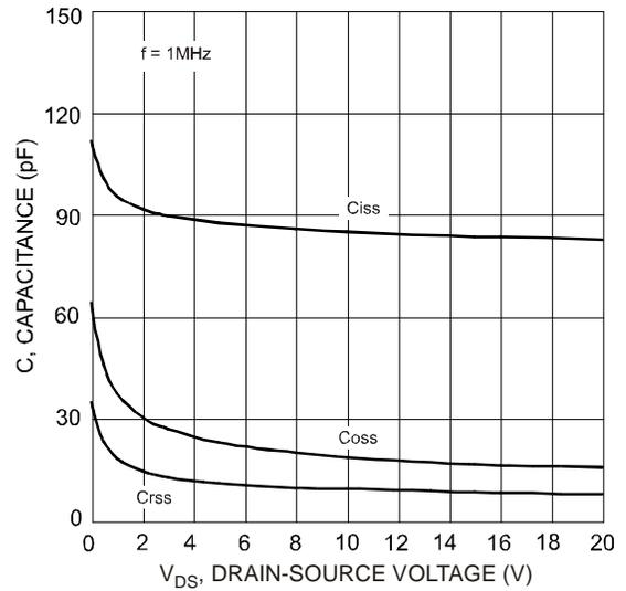
Fig. 10 Typical Capacitance
