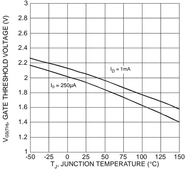
Figure 7 Gate Threshold Variation vs. Junction Temperature
