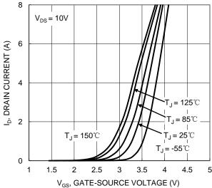
V<sub>GS</sub>, GATE-SOURCE VOLTAGE (V) Figure 2. Typical Transfer Characteristic
