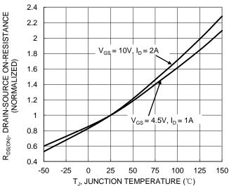
Figure 6. On-Resistance Variation with Junction Temperature
