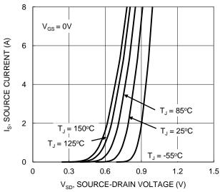
Figure 9. Diode Forward Voltage vs. Current
