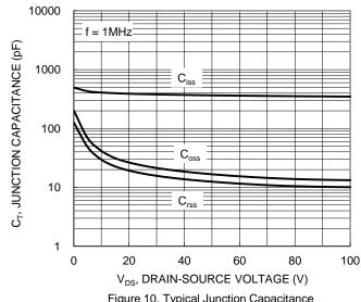
Figure 10. Typical Junction Capacitance
