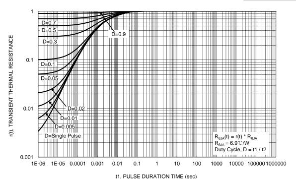
Figure 13. Transient Thermal Resistance
