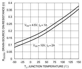
Figure 7. On-Resistance Variation with Junction Temperature
