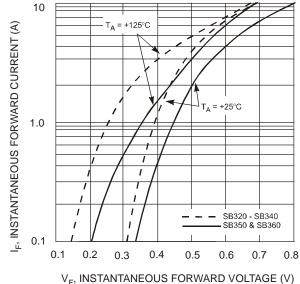
V<sub>F</sub>, INSTANTANEOUS FORWARD VOLTAGE (V Fig. 2 Typical Forward Characteristics
