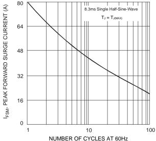
Fig. 3 Max Non-Repetitive Peak Forward Surge Current
