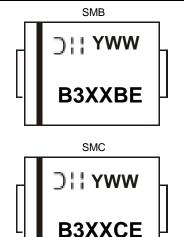
B3XXBE = Product Type Marking Code, ex: B320BE JII = Manufacturers' Code Marking YWW = Date Code Marking Y = Last Digit of Year (ex: 0 for 2020) WW = Week Code (01 to 53)
