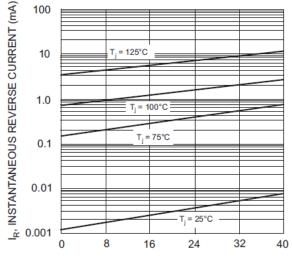
V<sub>R</sub>, INSTANTANEOUS, REVERSE VOLTAGE (V) Fig. 6 Typical Reverse Characteristics, SB520 - SB540
