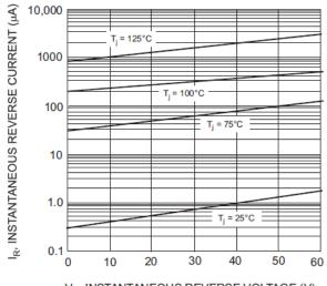
V<sub>R</sub>, INSTANTANEOUS REVERSE VOLTAGE (V) Fig. 7 Typical Reverse Characteristics, SB550 & SB560
