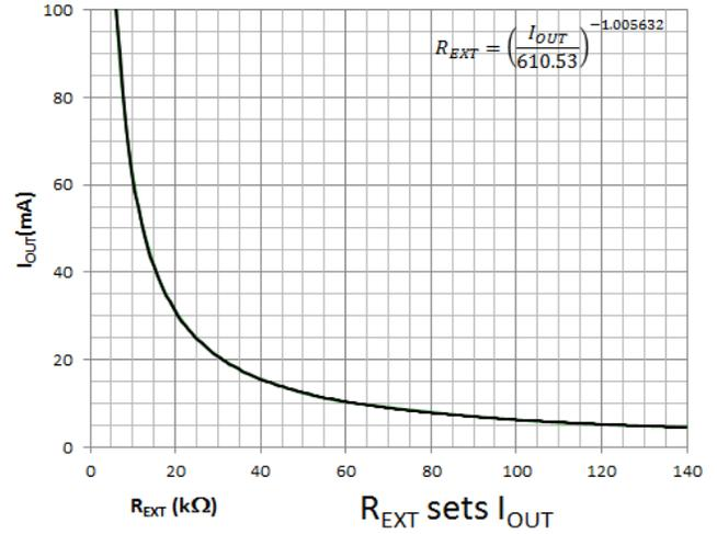
The LED current is set according to the resistor value which is connected to the REXT pin.
