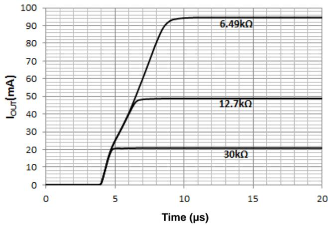
For  $R_{EXT} = 6.49k\Omega$ ,  $t_R = 14\mu s$  at  $-40^\circ C$ ,  $9\mu s$  at  $+25^\circ C$  and  $7\mu s$  at  $+110^\circ C$ .
