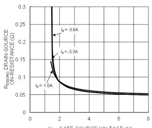
V<sub>os</sub>, GATE-SOURCE VOLTAGE (V) Figure 16 Typical Transfer Characteristic
