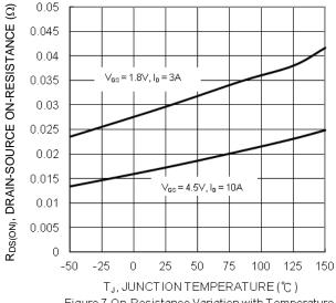
Figure 7 On-Resistance Variation with Temperature
