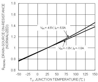
Figure 18 On-Resistance Variation with Temperature
