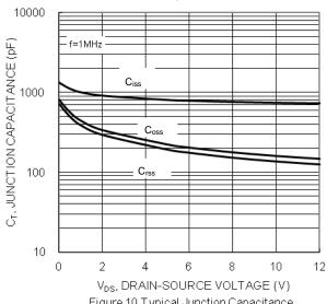
Figure 10 Typical Junction Capacitance
