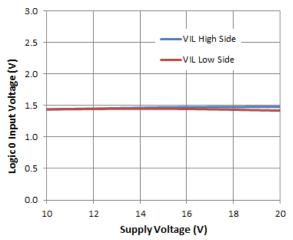
Figure 22. Logic O Input Voltage vs. Supply Voltage
