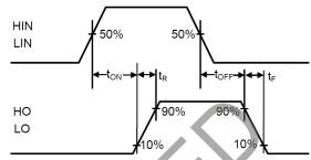
Figure 1. Input / Output Timing Diagram
