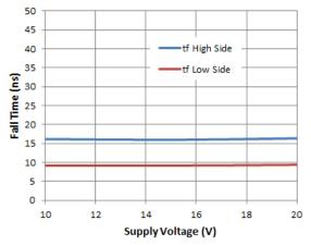
Figure 10. Fall Time vs. Supply Voltage
