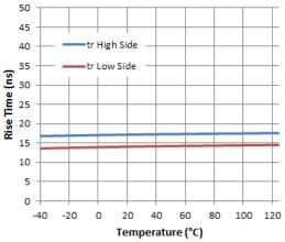
Figure 9. Rise Time vs. Temperature
