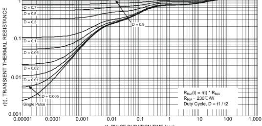
t1, PULSE DURATION TIME (sec) Fig. 2 Transient Thermal Resistance
