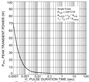
Fig. 1 Single Pulse Maximum Power Dissipation
