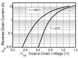
Source-Drain Diode Forward Voltage
