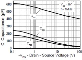
Capacitance v Drain-Source Voltage
