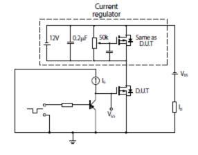
Gate charge test circuit
