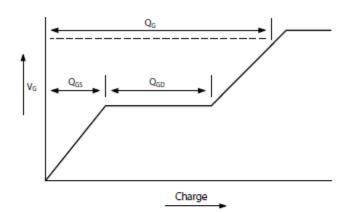
Basic gate charge waveform
