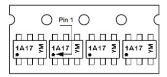
**ZXMP10A17E6QTAR**Rotate 180 degree of Pin 1 orientation in the carrier tape.
