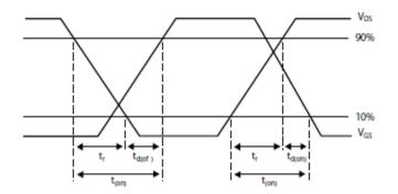
Switching time waveforms
