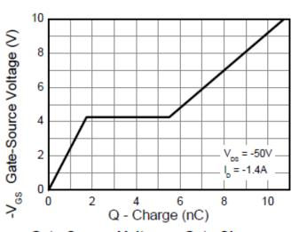
Gate-Source Voltage v Gate Charge
