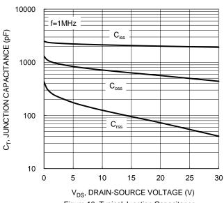
Figure 10. Typical Junction Capacitance
