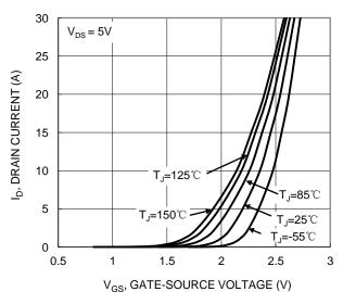
Figure 2. Typical Transfer Characteristic
