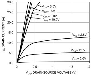
Figure 1. Typical Output Characteristic
