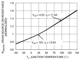
Figure 6. On-Resistance Variation with Junction Temperature
