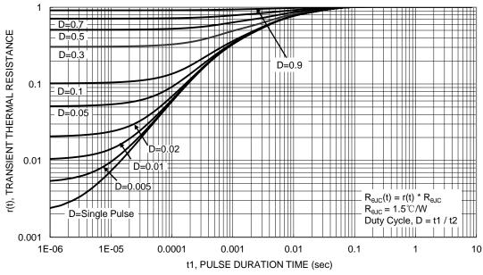
Figure 13. Transient Thermal Resistance
