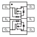
Top View Schematic and Pin Configuration
