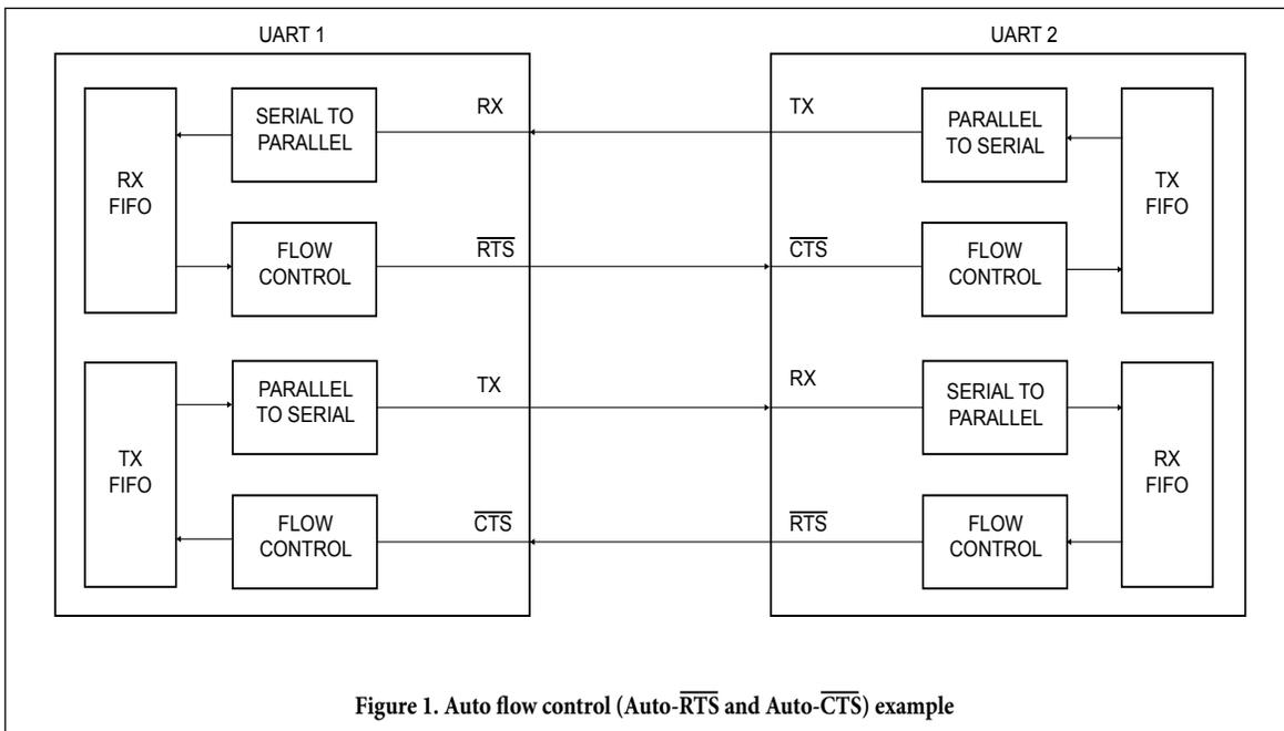
Figure 1. Auto flow control (Auto- $\overline{\text{RTS}}$  and Auto- $\overline{\text{CTS}}$ ) example
