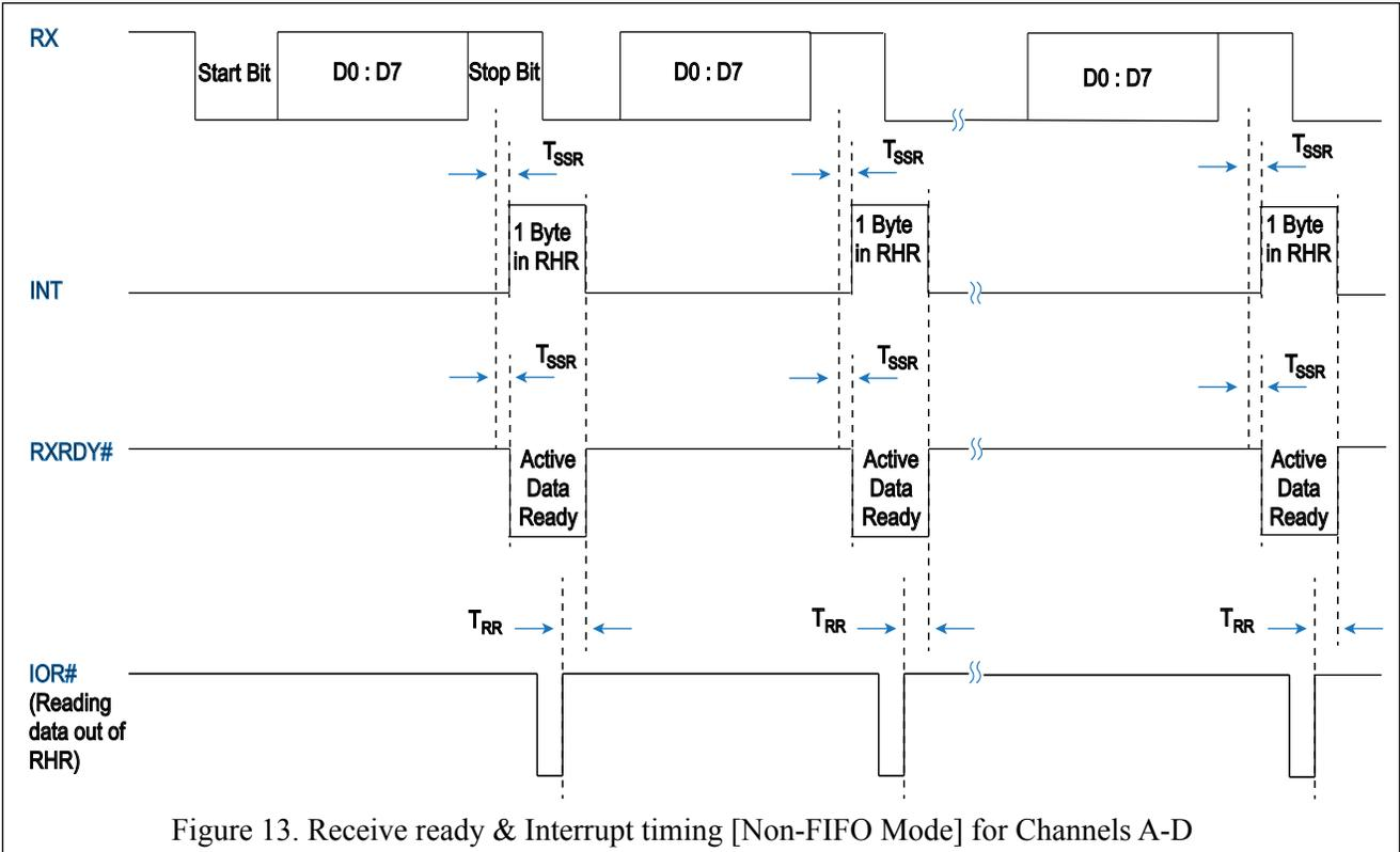
Figure 13. Receive ready & Interrupt timing [Non-FIFO Mode] for Channels A-D
