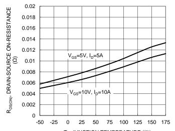
Figure 5. On-Resistance Variation with Temperature
