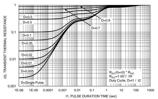
Figure 12. Transient Thermal Resistance
