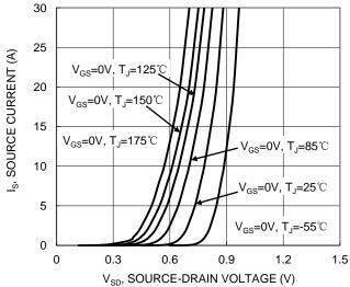
Figure 8. Diode Forward Voltage vs. Current
