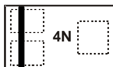
Top View Bar Denotes Gate and Source Side
