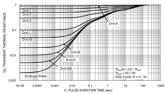
Figure 13. Transient Thermal Resistance
