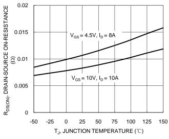
Figure 7. On-Resistance Variation with Temperature
