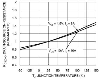
Figure 6. On-Resistance Variation with Temperature
