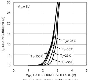
Figure 2. Typical Transfer Characteristic
