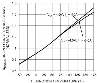
Figure 6. On-Resistance Variation with Temperature
