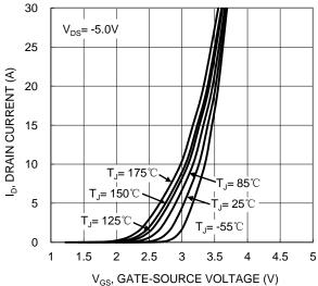
Figure 2. Typical Transfer Characteristic
