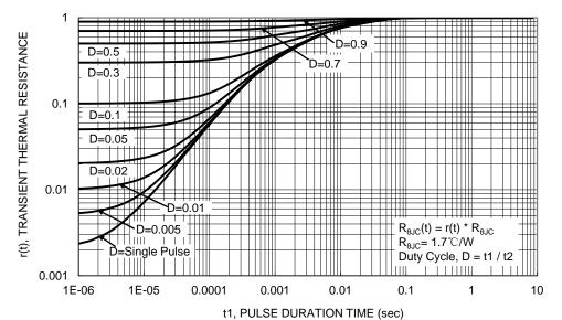
Figure 13. Transient Thermal Resistance
