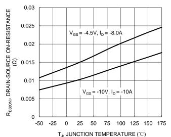
Figure 7. On-Resistance Variation with Temperature
