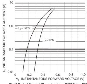
Fig. 2 Typical Forward Characteristics - B350Q thru B360Q
