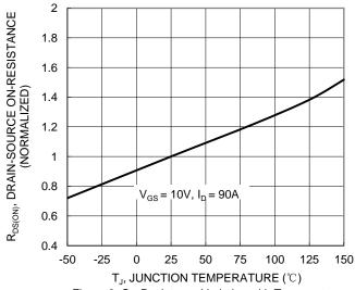
Figure 6. On-Resistance Variation with Temperature
