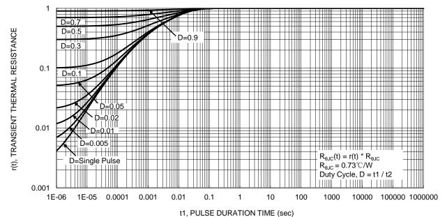
Figure 13. Transient Thermal Resistance
