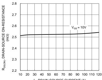
I<sub>D</sub>, DRAIN-SOURCE CURRENT (A) Figure 3. Typical On-Resistance vs. Drain Current and Gate Voltage
