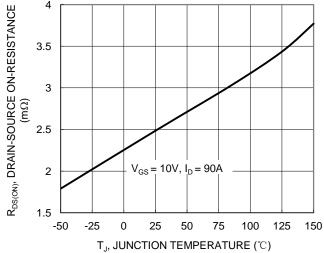
Figure 7. On-Resistance Variation with Temperature
