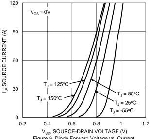
Figure 9. Diode Forward Voltage vs. Current
