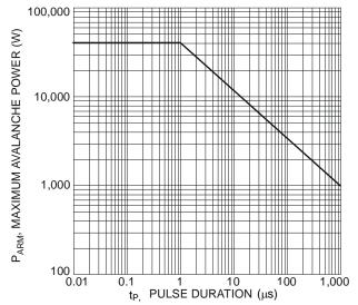
Figure 4 Maximum Avalanche Power Curve, Per Element
