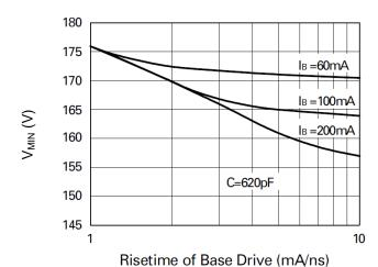
Minimum starting voltage as a function of drive current
