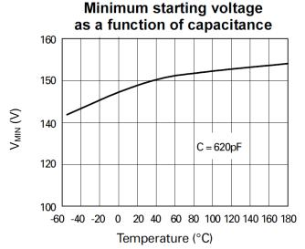
Minimum starting voltage as a function of temperature
