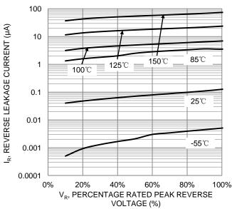
Figure 4. Typical Reverse Characteristics
