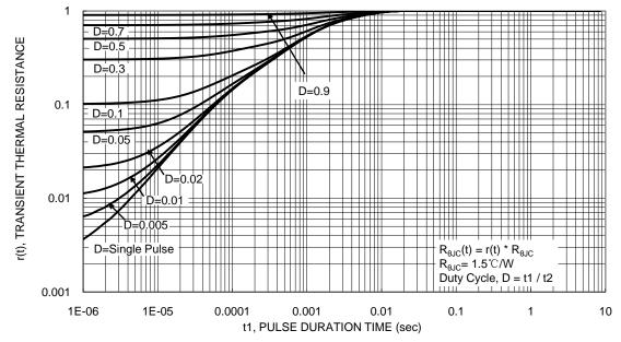
Figure 13. Transient Thermal Resistance
