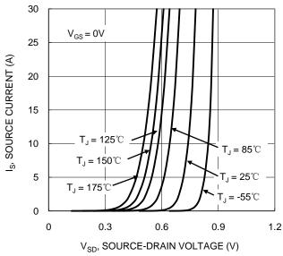
Figure 9. Diode Forward Voltage vs. Current
