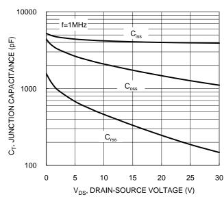
Figure 10. Typical Junction Capacitance
